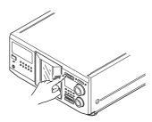
**3** Turn the JOG dial until you find the disc slot where you want to insert a disc, while checking the disc number (written beside every slot and also indicated in the small display).
